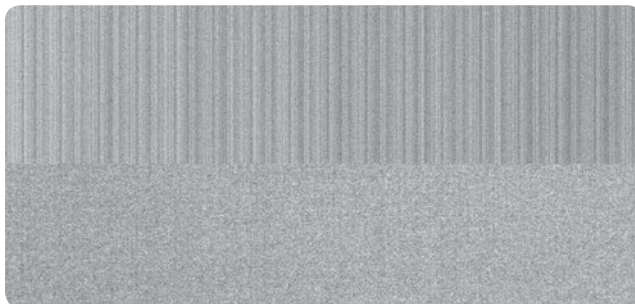
The top image shows the typical fixed pattern structures in the dark image of high speed CMOS image sensors, while the lower image shows the lower and more homogeneous noise in the dark image of a pco.dimax.
