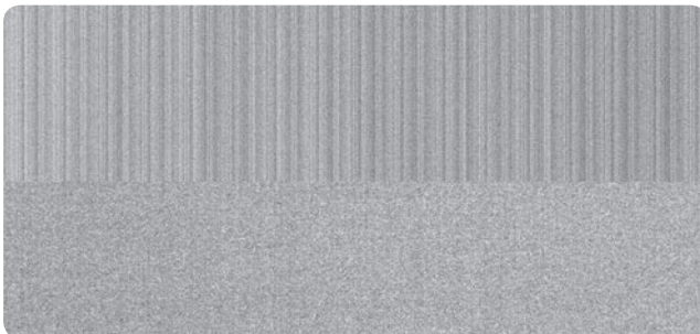
The top image shows the typical fixed pattern structures in the dark image of high speed CMOS image sensors, while the lower image shows less and more homogeneous noise in the dark image of a pco.dimax.
