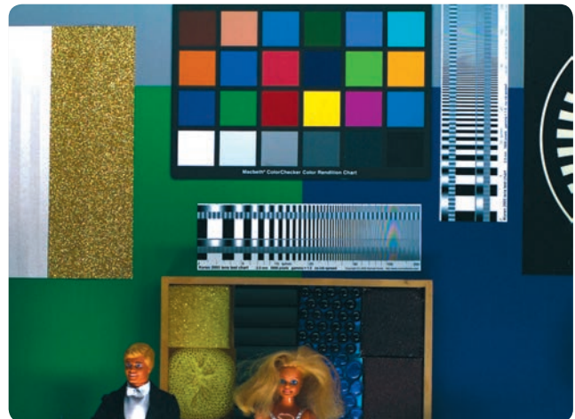
A typical test image with color checker, MTF test charts and challenging structures obtained with a color pco.dimax.
