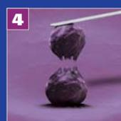
4 The cell resists the attempt of removing it from the surface if it adheres to the target. Therefore the cantilever bends noticeably, which is measured by a detector.
