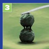
3 After a user-defined reaction time the cell on the cantilever is separated from the substrate cell by retracting the cantilever in vertical direction (z-axis) through a piezo actuator.
