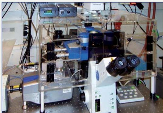
CellHesion® 200 mounted on Olympus base with incubator
