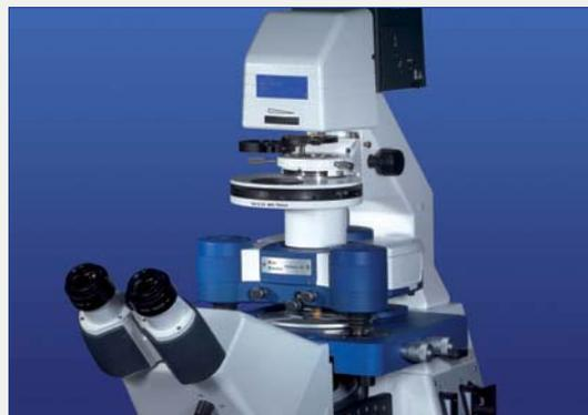
CellHesion<sup>®</sup> 200 setup on Zeiss Axio Observer
