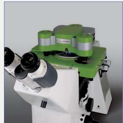
The ForceRobot®300 mounted on a Zeiss AxioObserver inverted optical microscope. It is compatible with all major research-level inverted optical microscope platforms, and all the stages can also be used unmounted for stand-alone operation.
