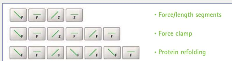
*RampDesigner™ schematic. Different segments can be freely combined in an intuitive interface, which gives complete flexibility in creating and reloading custom force curve settings.*
